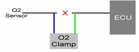
The use of bullet-style crimp connectors is suggested for the blue, green and white wires to allow for easy installation and removal of the  $O_2$  clamp. Connections to +12 and ground can be made with T-taps (also called vampire taps) to attach to the existing wires which supply the ECU / EMU. When finished, re-connect the battery cable.
